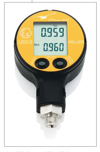
Developed and designed in line with practical requirements, this manometer is available for prompt delivery with four measurement ranges of -1...3 bar to 0...700 bar. The standard design already offers IP65 as the housing protection class. The optional protective cover enables the LEO 2 to operate reliably outdoors in all weather conditions. This instrument is also available in an Exia ATEX approved version compliant with 94/9/EC (ATEX 100a).
