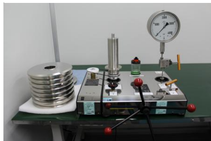
Europascal Hydraulic DWT-BH2-4000 Max. 4,000bar
