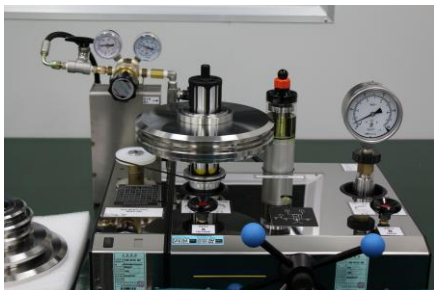
Europascal Pneumatic DWT-BA2-70 Max. 70bar
