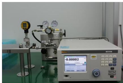
Fluke Controller PPC4EX-7M 7MPa & 700kPa / 0.005% of F.S
